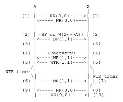
(1) The protection domain is operating without any defect, and the working entity is used for delivering the normal traffic.
