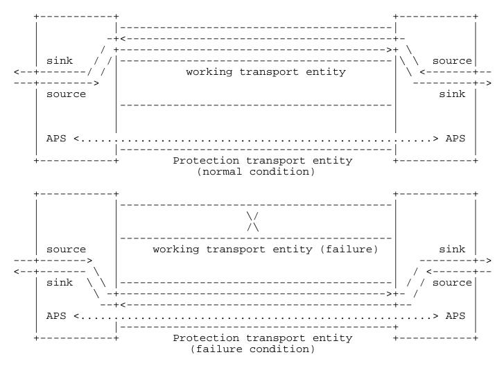
Figure 3 1:1 Bidirectional Linear Protection Switching
