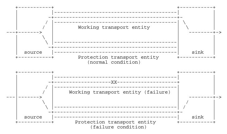
Figure 1 1+1 Unidirectional Linear Protection Switching
