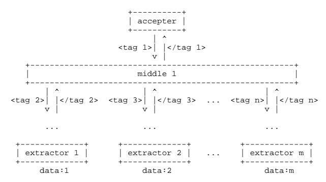
Figure 2: DFA Architecture of Data Extractor
