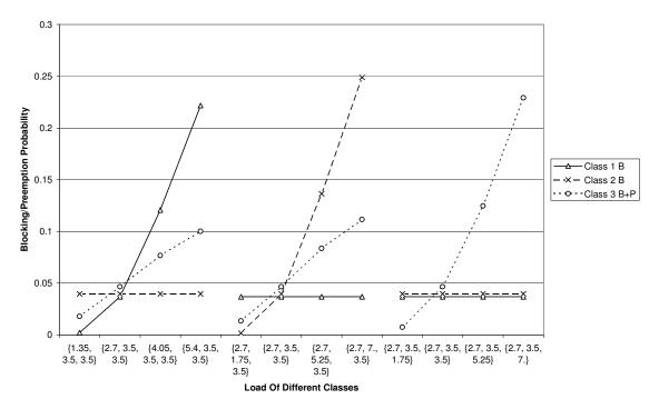
Figure 6. Maximum Allocation, with partial preemption (1+2 on 3).
