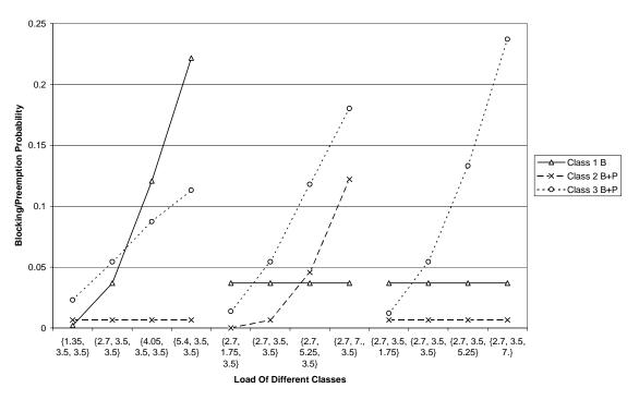
Figure 1bis. Maximum Allocation (6, 9, 15), with full preemption.
