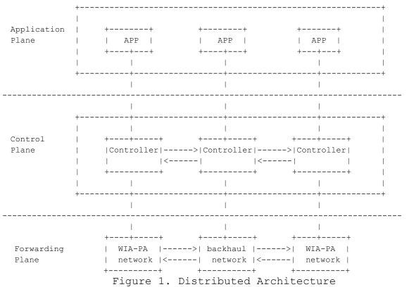
In distributed architecture, controller can exchange different network topologies and the accessibility of information by east-west interface, and each controller can establish a global network topology. From a global network perspective, each controller is equal, thus it can serve as a server role as well as the ability to start deterministic crossnetwork transmission task.
