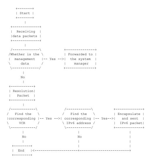
Figure 4. The process of protocol conversion in gateway
