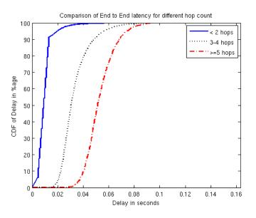
Figure 25: Comparison of packet latency for different hop count in RPL.
