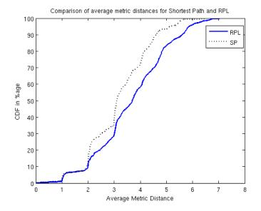
Figure 22: Comparison of path ETX metric for RPL and ideal shortest path in home routing.
