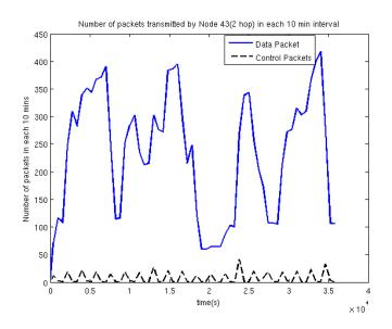
Figure 11: Amount of data and control packets transmitted for node 43.
