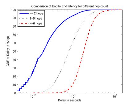
Figure 29: End-to-end packet delivery latency for different hop count
