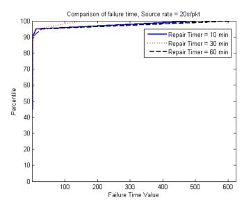
Figure 17: CDF: Loss of connectivity for different DAG repair timer values for gloabal+local repair, packet rate 20/s.
