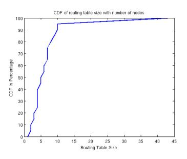
Figure 7: CDF of routing table size with respect to number of nodes.
