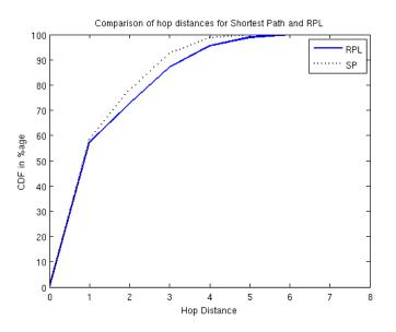
Figure 21: Comparison of end-to-end hop distance for RPL and ideal shortest path in home routing.
