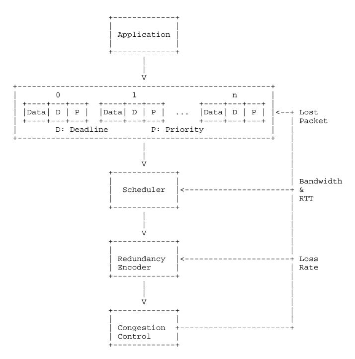
Figure 1: The Architecture of DTP
