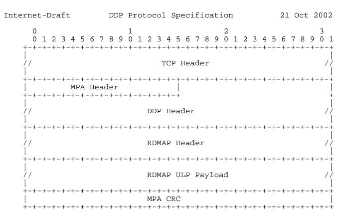
Figure 2 MPA, DDP, and RDMAP Header Alignment
