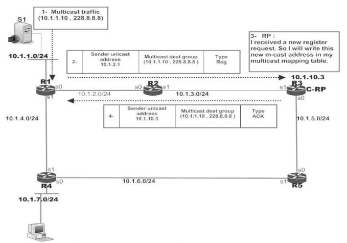
Figure 5 source communication with the RP
