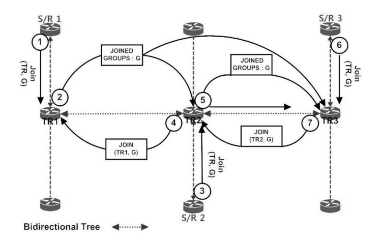
Figure 56 Bidirectional Tree formation with ANYCAST TR Address
