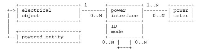
Figure 19: Basic Information Model of the PSU Layer
