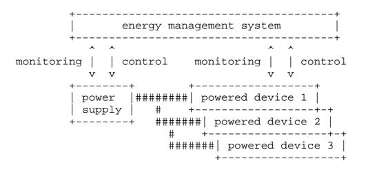
Figure 4: Multiple Powered Devices Supplied by Single Power Line
