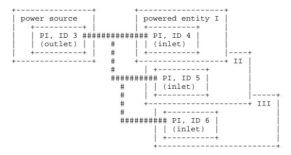
Figure 9: PSU Layer for a Single PS Supplying Multiple PEs. The corresponding PSU layer data model is shown by Figure 10.
