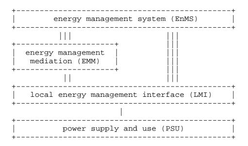
Figure 1: Layers of the Energy Management Reference Model
