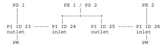
Figure 18: Relationships between Cascaded Power Sources
