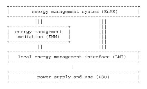
Figure 6: Layers of the Energy Management Reference Model
