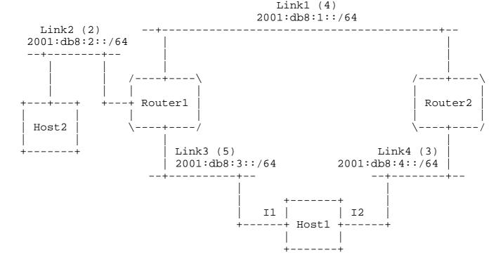
The figure shows two routers (Router1, Router2) and two hosts (Host1, Host2). Theses nodes are connected to each other through 4 links (Link1, Link2, Link3, Link4). The values in brackets represent the corresponding link costs. Also, Host1 is a multiple interfaces device: it is connected to Link3 via its network interface I1 and to link4 via its network interface I2.
