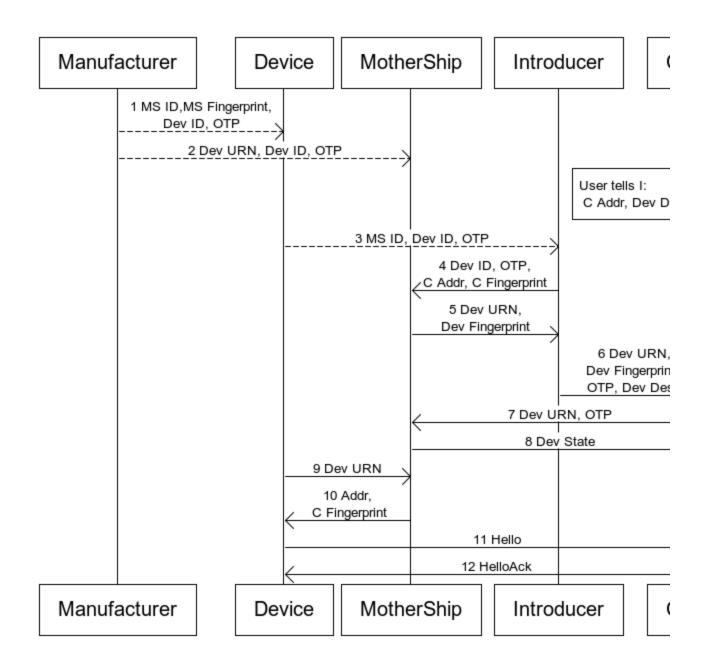
When the Device is built, it needs to be assigned a globally unique URN, a Dev ID, and a MotherShip. A single manufacturer MAY operate many MotherShips as each one can only support 16 million Devices. A perfectly reasonable way to generate the Dev ID is to use the least significant 32 bits of the Device URN. The Device needs to be programmed with the IP address and port of the MotherShip along with the fingerprint of the public key that the MotherShip will use in the DTLS CoAP exchange.
