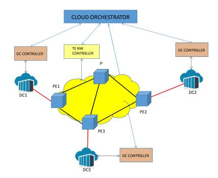
Figure 5 - Data Center Interconnection Use Case
