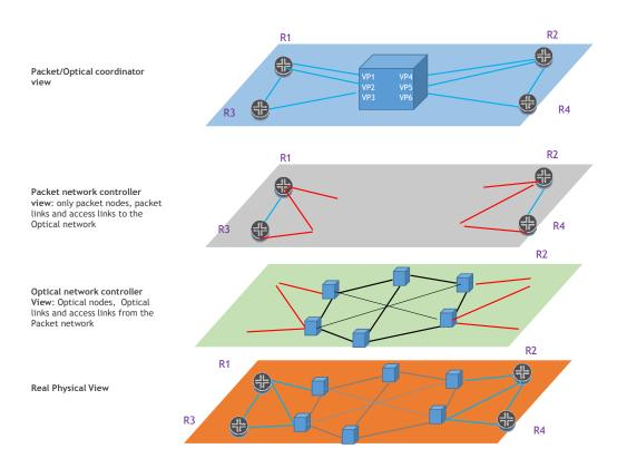
Figure 2 - Packet and Optical Topology Abstractions
