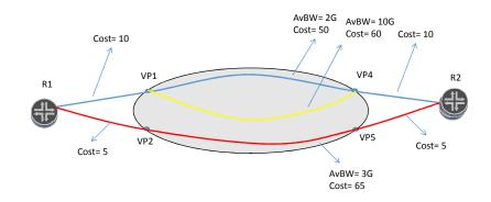
Figure 6 - Packet/Optical Path Computation Example with multiple choices
