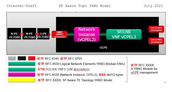
Figure 11: uCPE Service Functions topology (simple)
