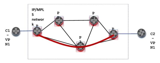
Figure 2: L3 VPN with delay constraints
