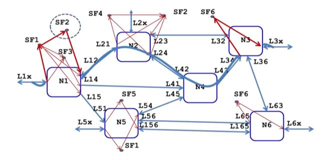
Figure 4: SFC recovery: SF2 on node NE1 fails
