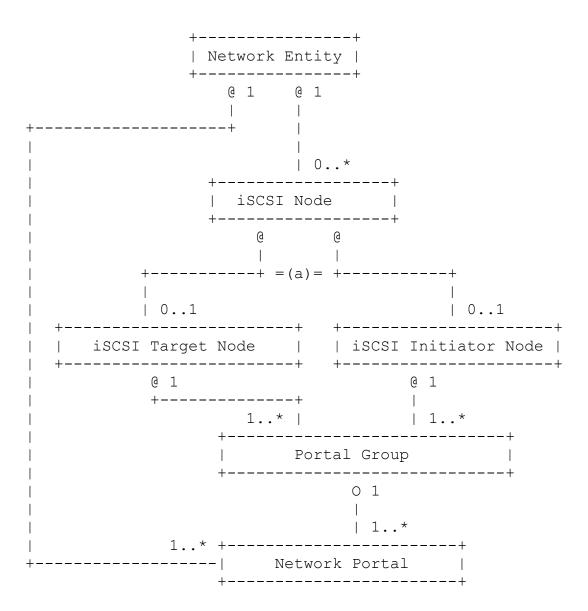
(a) Each instance of an iSCSI Node class MUST contain one iSCSI Target Node instance or one iSCSI Initiator Node instance, or both.
