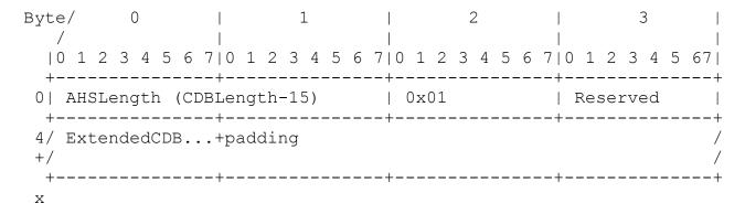
This type of AHS MUST NOT be used if the CDBLength is less than
