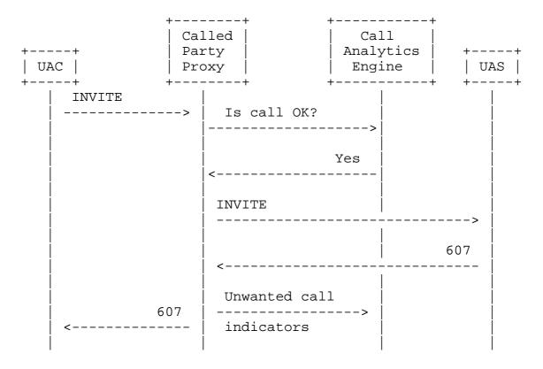
Figure 2: Unwanted (607) Ladder Diagram
