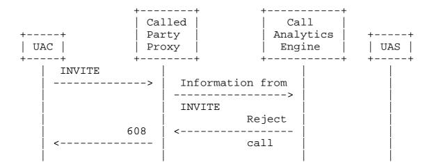
Figure 4: Rejected (608) Ladder Diagram
