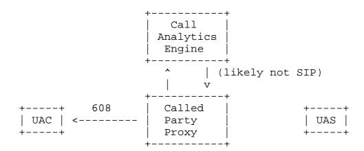
Figure 3: Rejected (608) Call Flow
