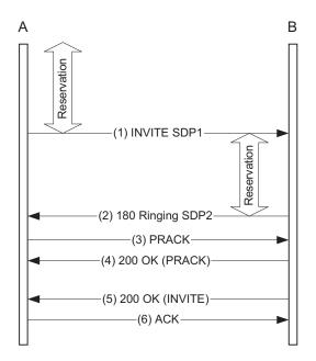
Figure 4: Example using the segmented status type
