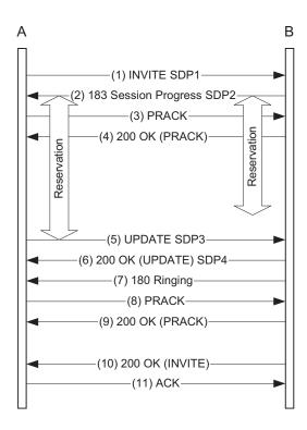
Figure 2: Example using the end-to-end status type
