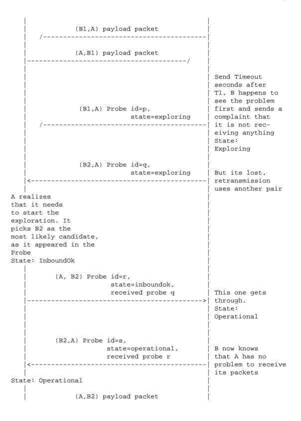
The next example shows when the failure for the current locator pair is in the other direction only. A has addresses Al and A2, and B has addresses Bl and B2. The current communication is between Al and Bl, but A's packets no longer reach B using this pair.
