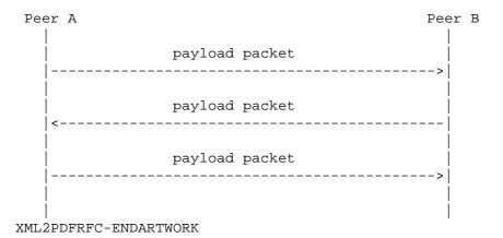
The third example is the first one that involves an actual REAP message. Here the hosts communicate in just one direction, so REAP messages are needed to indicate to the peer that sends payload packets that its packets are getting through:
