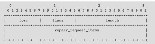
Figure 18: NORM Repair Request Format
