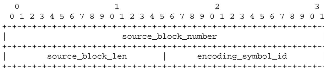
*Small Block, Systematic Code ("fec\_id" = 129) "fec\_payload\_id" Format*
