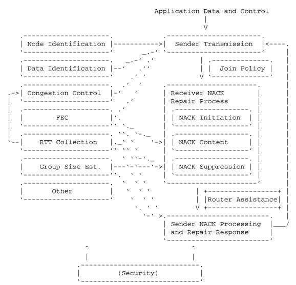
Fig. 1 - NACK-based Reliable Multicast Building Block Framework
