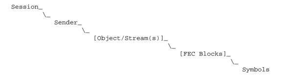
Fig. 2: Reliable Multicast Data Content Identification Hierarchy
