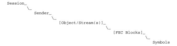
Fig. 2: NORM Data Content Identification Hierarchy
