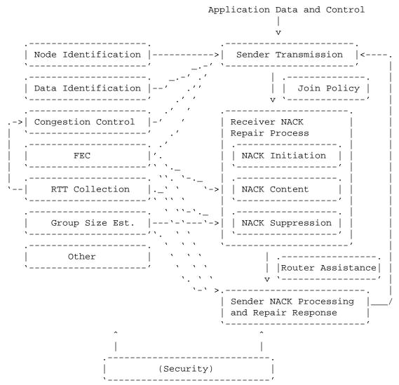
Fig. 1 - NORM Building Block Framework
