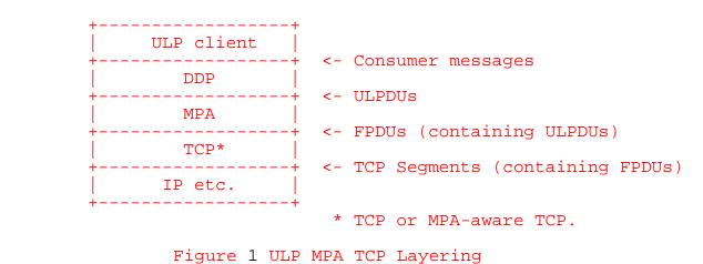
MPA is described as an extra layer above TCP and below DDP. The operation sequence is:
