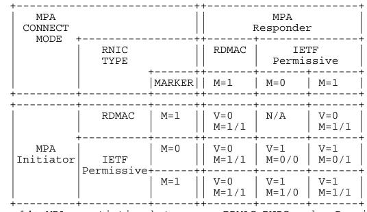
Figure 14: MPA negotiation between an RDMAC RNIC and a Permissive IETF RNIC.
