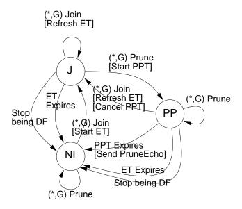
Figure 1: Downstream group per-interface state-machine
