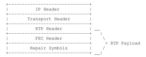
Figure 9: Format of repair packets
