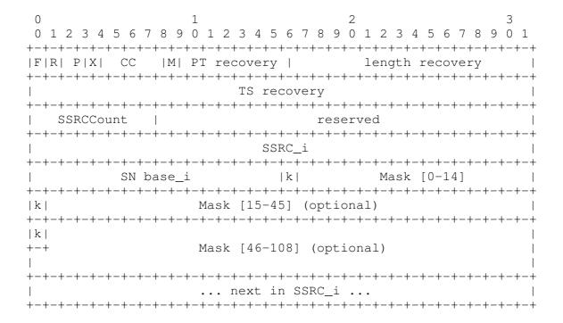
Figure 10: Format of the FEC header
