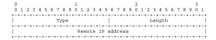
Figure 1: Link-Overload sub-TLV for OSPFv2
