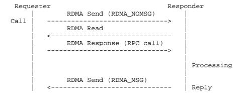
An RPC-over-RDMA transaction using a Long Reply:
