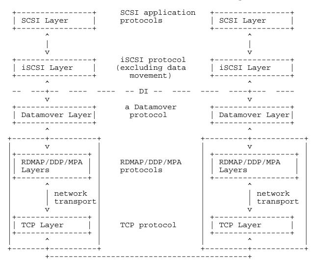
Figure 1 Datamover Architecture diagram, with the RDMAP example
