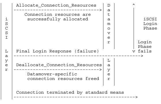
Figure 5 A failed iSCSI login on target
