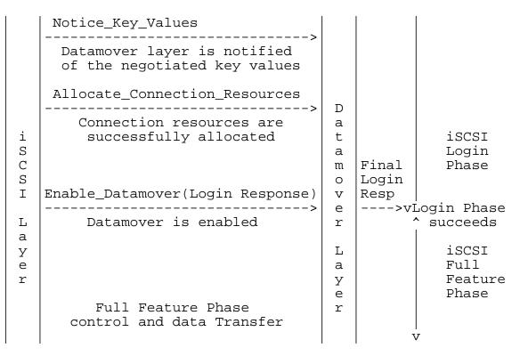
Figure 3 A successful iSCSI login on target
