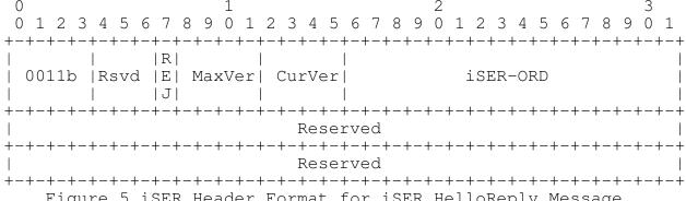
Figure 5 iSER Header Format for iSER HelloReply Message
