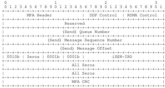
Figure 6 SendSE Message containing an iSER Hello Message
