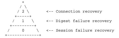
The following table lists the error recovery capabilities expected from the implementations that support each error recovery level.
