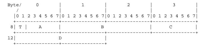
The T field identifies the format and usage of A, B, C, and D as indicated below:
