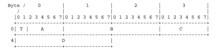
The T field identifies the format and usage of A, B, C & D as indicated bellow:
