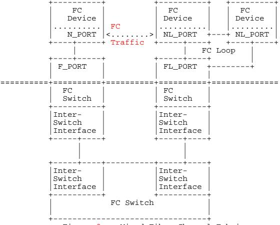
Figure 3 -- Mixed Fibre Channel Fabric
