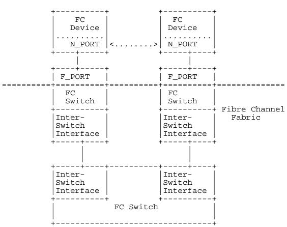
Figure 2 -- Multi-Switch Fibre Channel Fabric
