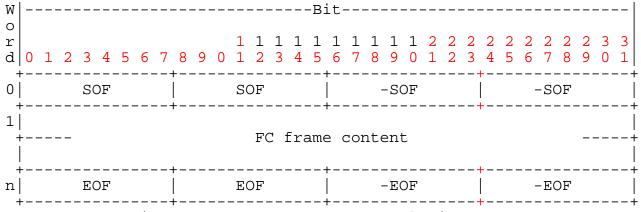
Figure 17 -- FC Frame Encapsulation Format
