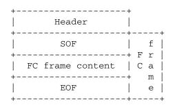
Fig. 1 - FC frame Encapsulation
