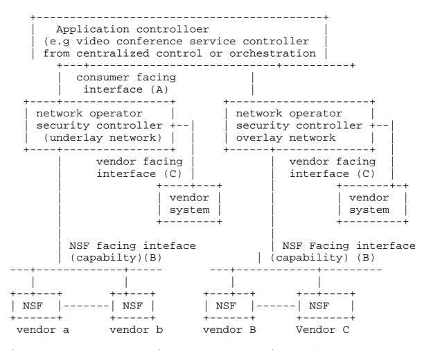
Figure 5: I2NSF Preventing DDoS Attacks in Overlay Networks.
