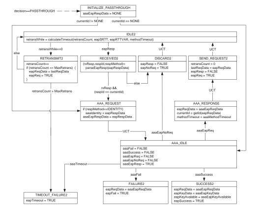
Figure 7: EAP Full Authenticator State Machine (Part 2)
