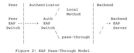
The Full/Pass-Through state machine allows a NAS or Edge Device to pass EAP Response messages to a Backend Server where the Authentication Method resides. This paper includes a state machine for the EAP authenticator that supports both local and pass-through methods as well as a state machine for the backend authenticator existing at the AAA server. A simple "Standalone" authenticator is also provided to show a basic, non-pass-through authenticator's behavior.
