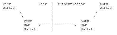
Figure 1: EAP Switch Model
