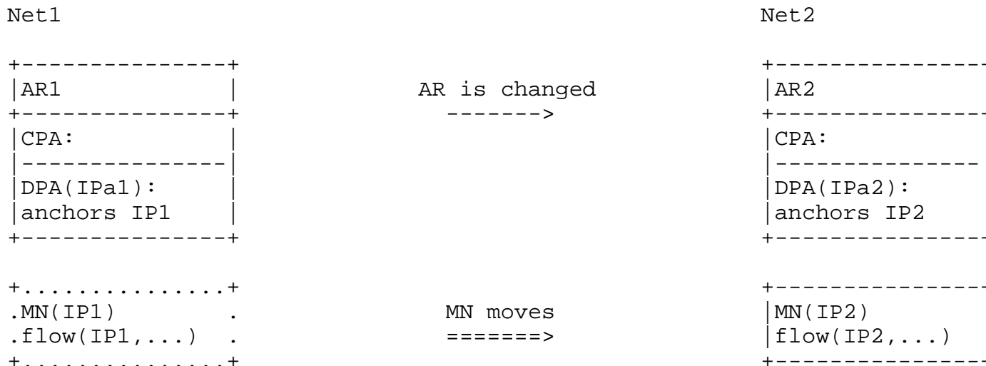
Figure 5. Changing to the new IP prefix/address. MN running a flow using IP1 in a network Net1 changes to running a flow using IP2 in Net2.
