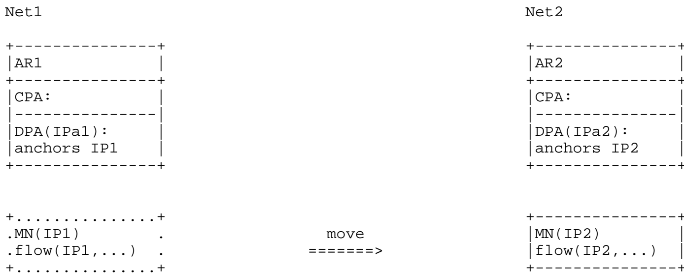
Figure 5. Changing to the new IP prefix/address. MN running a flow using IP1 in a network Net1 changes to running a flow using IP2 in Net2.
