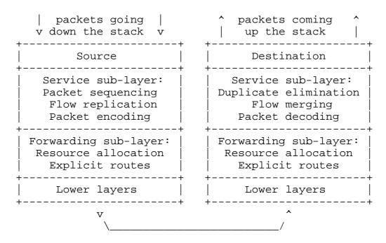
Figure 2: DetNet data plane protocol stack
