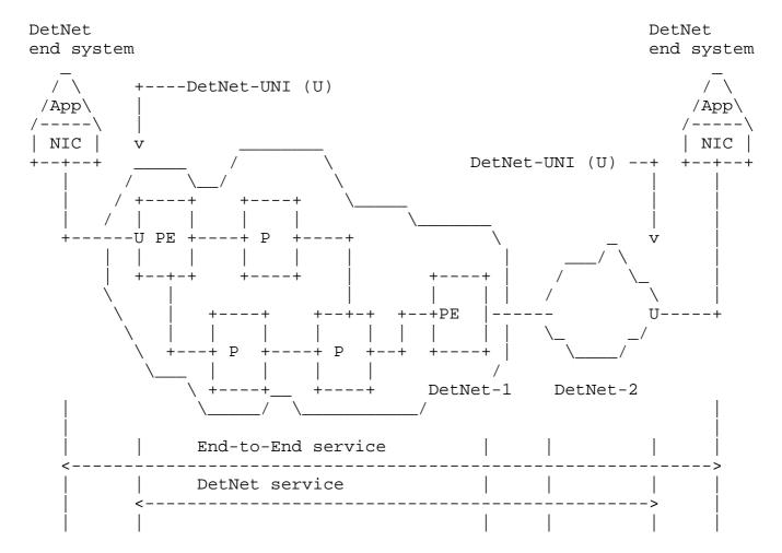
Figure 5: DetNet Service Reference Model (multi-domain)
