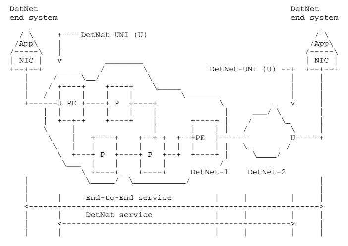
Figure 5: DetNet Service Reference Model (multi-domain)
