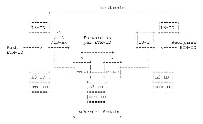
Figure 10: IP nodes interconnected by an Ethernet domain
