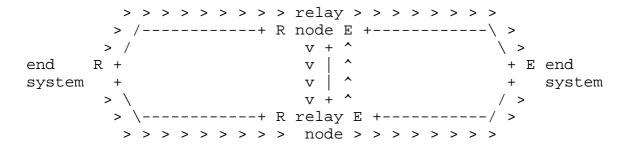
Figure 1: Packet replication and elimination
