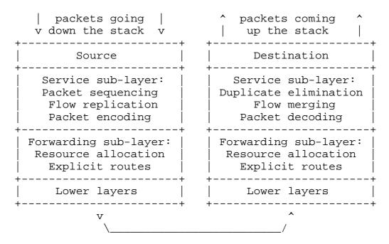
Figure 2: DetNet data plane protocol stack
