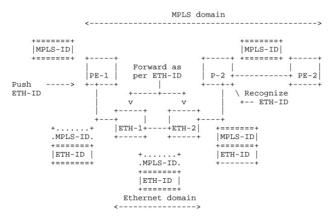
Figure 11: MPLS nodes interconnected by an Ethernet domain
