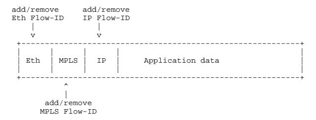
Figure 9: Packet with multiple Flow-IDs
