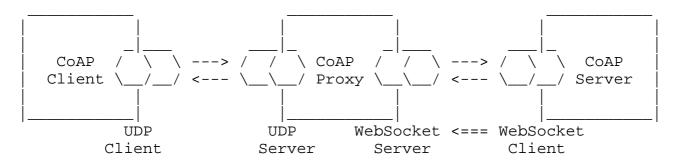
Figure 11: CoAP Client (UDP client) accesses CoAP Server (WebSocket client) via a CoAP proxy (UDP server/WebSocket server)
