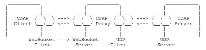
Figure 10: CoAP Client (WebSocket client) accesses CoAP Server (UDP server) via a CoAP proxy (WebSocket server/UDP client)
