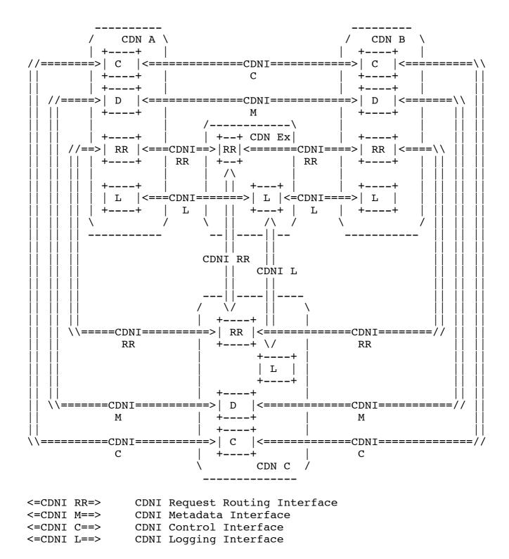
Figure 14: CDNI Deployment Model: CDN Exchange
