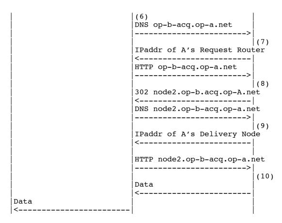
Figure 3: Message Flow for Iterative HTTP Redirection
