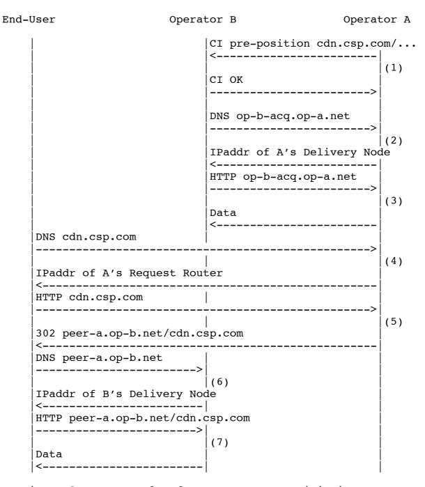
Figure 8: Message Flow for Content Pre-Positioning
