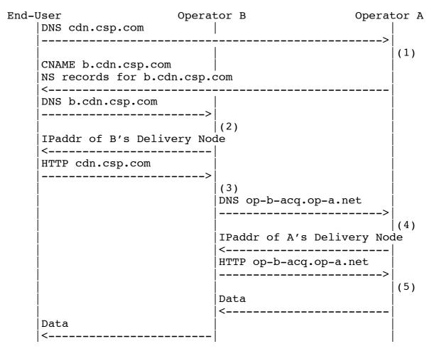
Figure 5: Message Flow for DNS-based Redirection
