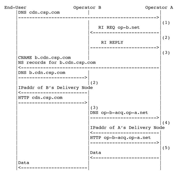
Figure 6: Message Flow for Dynamic Footprint Discovery
