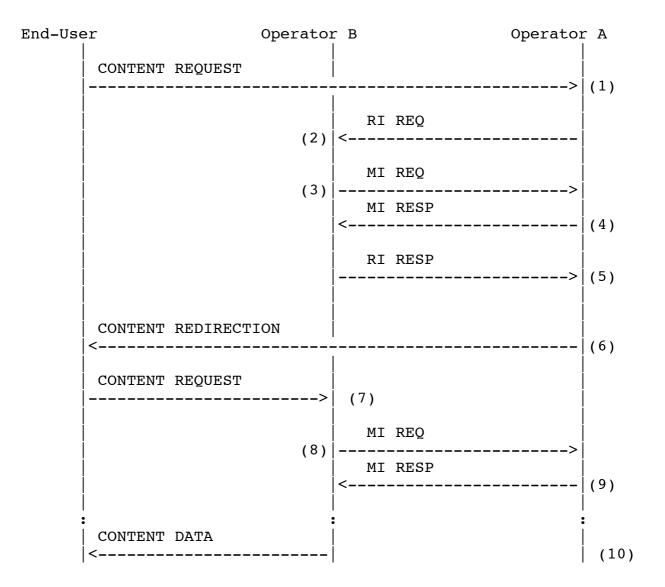
Figure 10: Message Flow for Synchronous CDNI Metadata Acquisition The steps illustrated in the figure are as follows:
