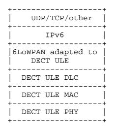
Figure 3: IPv6 over DECT ULE Stack
