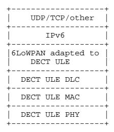
Figure 3: IPv6 over DECT ULE Stack
