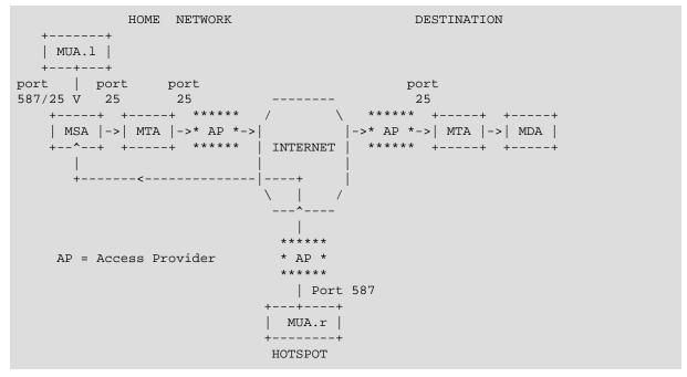
Figure 1: Example of Port 587 Usage Via Internet
