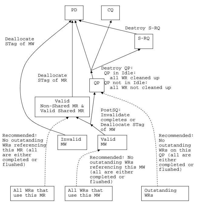
Figure 3 - Resource Destruction Dependency Diagram
