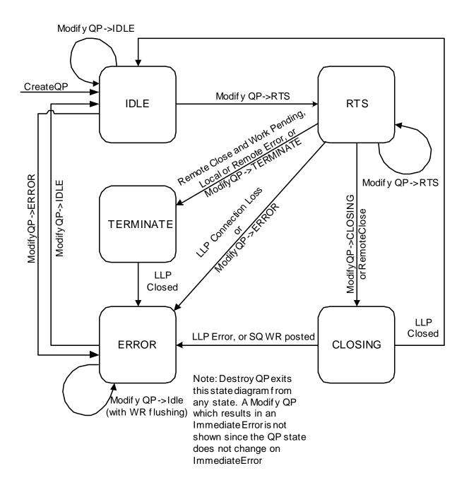
Figure 6 - QP State Diagram
