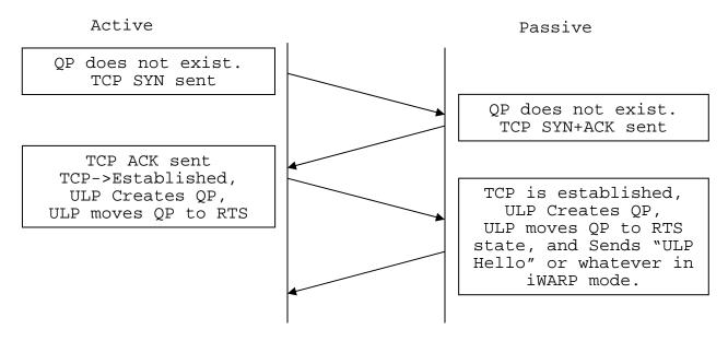
Figure 39 - Connection Initialization at LLP Startup (using TCP)
