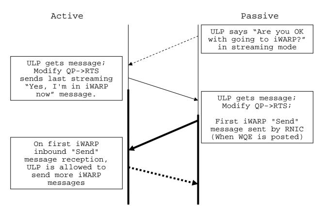
Figure 14 - Connection Initialization after LLP Startup
