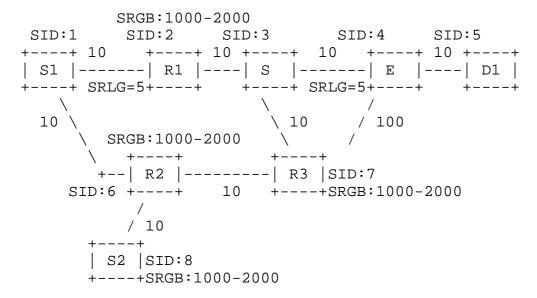
Figure 6: Sample Network with SRLG links
