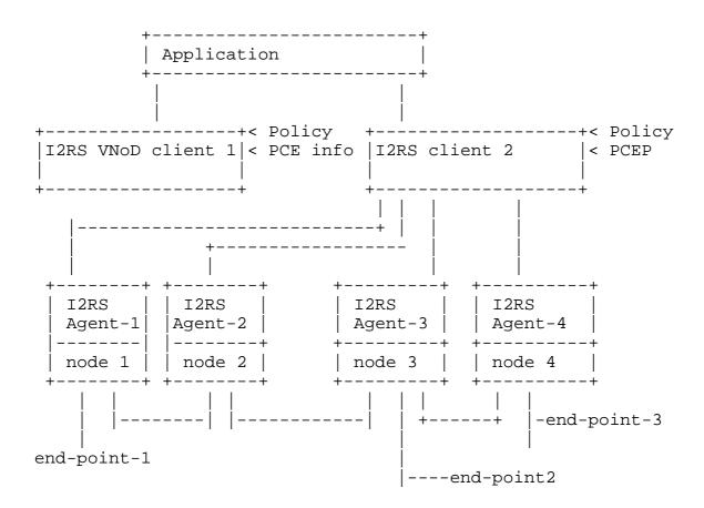
This topology shares some configuration needs with the central membership computation for MPLS VPNs from (draft-white-i2rs-usecases) but the mechanisms are not specific to MPLS VPNS.
