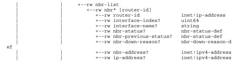
Figure 2 draft-i2rs-wang-ospf-dm-00 ospf-nbr-list structure
