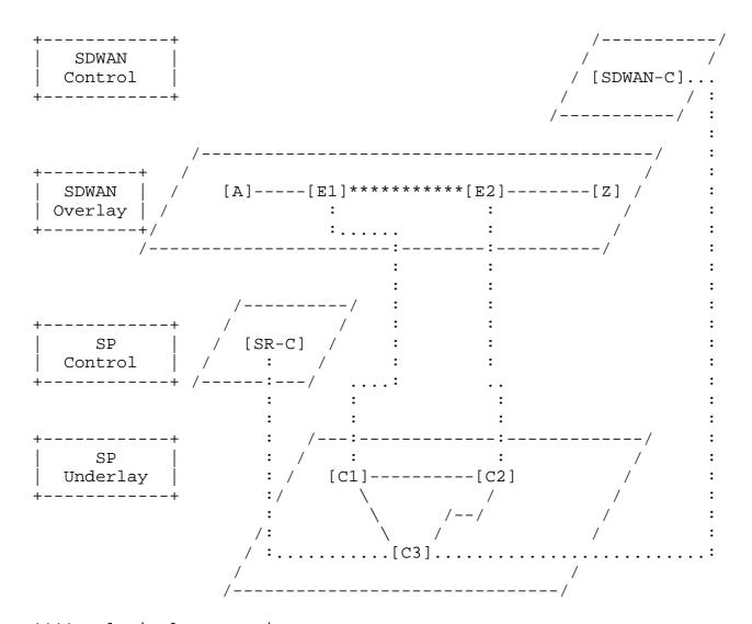
\*\*\*\* = logical connection :... = physical connection, between layers /-- = physical connection, within a layer
